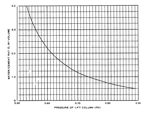
Figure 4. Pressure of neat cement grout
