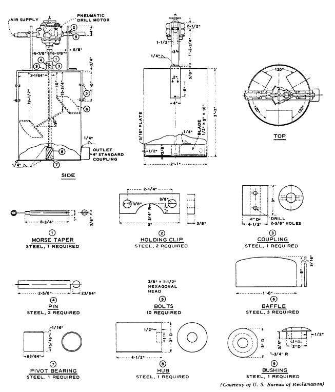
Figure 9. Central Valley-type grout mixer, 8-cu-ft capacity
