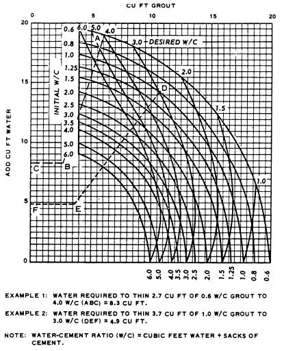
CEMENT. FOR DETERMINATION OF QUANTITY OF WATER TO ADD, LAY STRAIGHTEDGE FROM POINT OF INTERSECTION OF INITIAL AND DESIRED WATER-CEMENT RATIO CURVES TO POINT 0 AT LOWER LEFT-HAND CORNER OF CHART. READ AMOUNT OF WATER TO ADD ON LEFT SIDE OF CHART OPPOSITE POINT WHERE STRAIGHTEDGE INTERSECTS VERTICAL LINE REPRESENTING CUBIC FEET OF GROUT TO BE THINNED.
