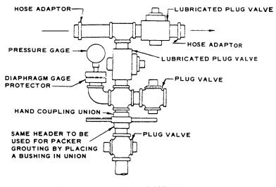
NOTE: ALL PIPE AND FITTINGS ARE 1-1/2" SIZE. PLUG VALVES TO BE USED THROUGHOUT FOR PRESSURES ABOVE 250 PSI. GROUT HOSE TO BE 1-1/2" WITH SCREW-TYPE COUPLINGS.
