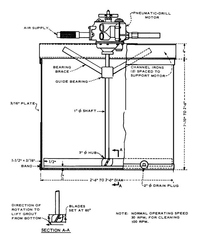
Figure 12. Grout agitator
